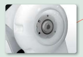
BXR spline type for holding arms. Saves space with slim design and greatly reduces drag wear by using light rotor.
