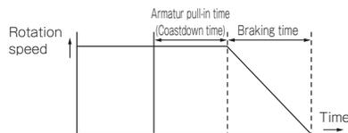
When brakes are used for long periods of time, they wear, air gaps grow, and it becomes impossible to pull in the armature even when the coil is excited. If re-adjustment becomes necessary, adjust the air gap as described in the maintenance and inspection section of the operating manual.
