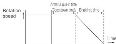
The time required from cutting off the power supply of a BMS model brake motor to stopping of the load is the braking time  $t_{ab}$  found with the above equation plus the armature release time.
