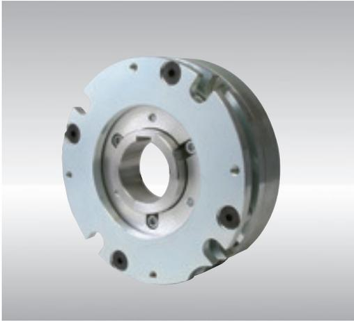
This is a large version of the BXW with static friction torque of 300 N·m. Backlash is kept extremely small by locking the rotor hub to the rotor via a disc spring.
