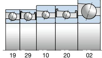
As shown in the figure above, for identical bore diameters, the bearings' outside diameter and width increase in the order 19– 29– 10– 20– 02 Series as expressed by the dimension series codes.
