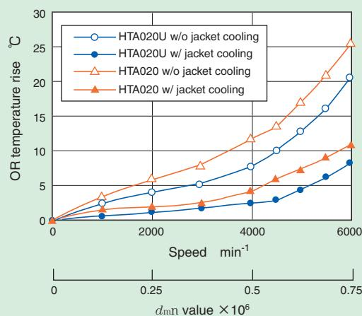
Fig. 11.7 Comparison of temperature rise (Grease,  $\alpha=40^\circ$ )
