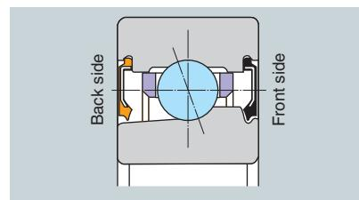
Fig. 9.9 High-speed grease-lubricated sealed angular contact ball bearings
