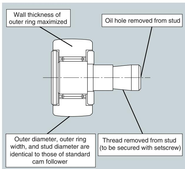
Fig. 14-1 Schematic of NTN pallet changer cam follower
