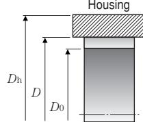
Fig. 6.17 Fit between outer ring and housing
