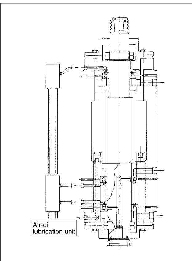
Fig. 9.16 Test rig for measuring temperature rise
