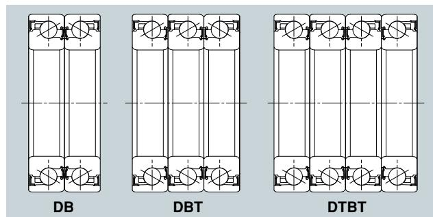
Fig. 13.2 Bearing arrangement
