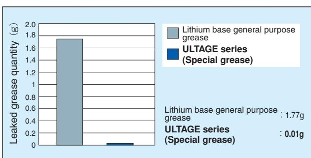
**Fig. 13.9 Grease leakage****② Duplex angular contact ball bearings HT series**
