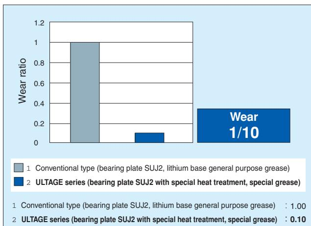
**Fig. 13.6 Ratio of fretting corrosion while rolling**
