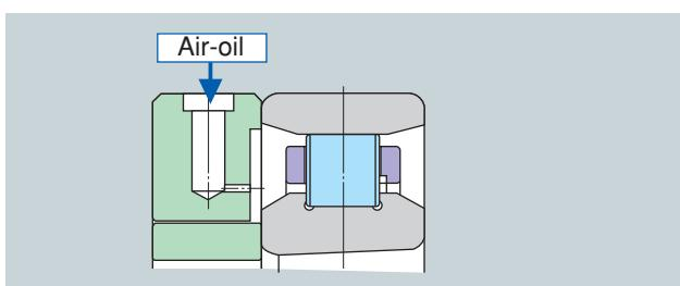
Fig. 8.9 Current bearing N10HS type
