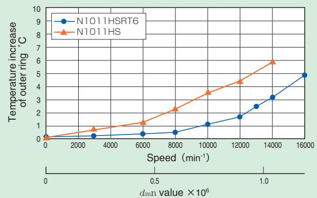
Fig. 10.12 High-speed test results (grease lubrication with outer case cooling)
