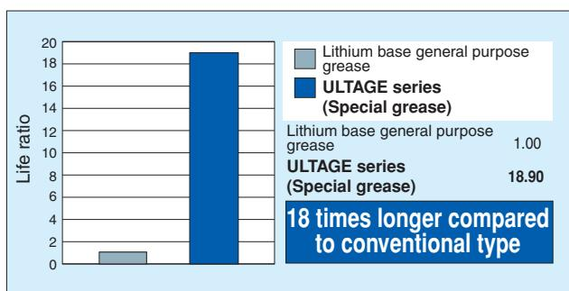
**Fig. 13.8 Grease life ratio****(5) Grease leakage test**
