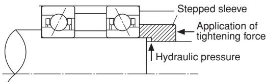
**Fig. 6.7** Tightening with stepped sleeve
