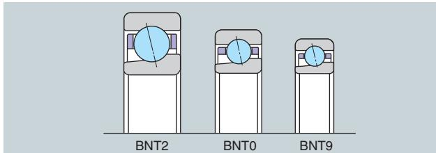
Fig. 9.7 High-speed angular contact ball bearings for grinding machines/motors
