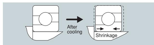
**Fig. 6.6 Cooling after mounting by heating bearings**
