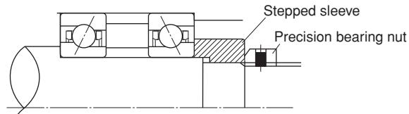
**Fig. 6.8** Tightening with stepped sleeve + precision bearing nut
