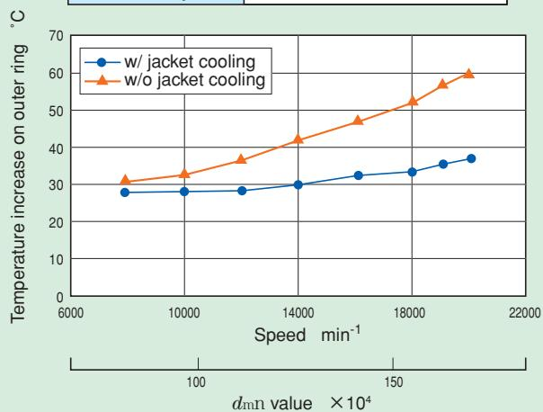
Fig. 5.6 Variation in bearing temperature depending on presence/absence of jacket cooling (angular ball bearing)
