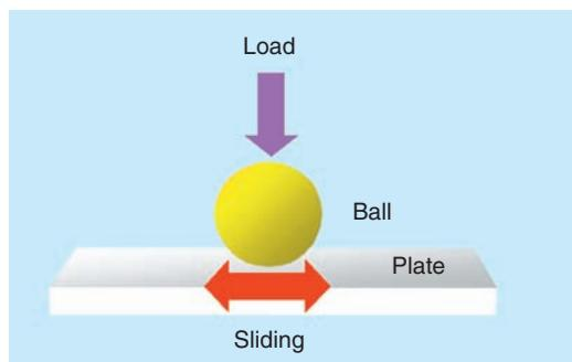
Fig. 13.3 Fretting resistance test (sliding)
