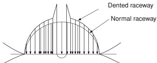
Fig. 3.4 Contact surface pressure distribution resulting from dent
