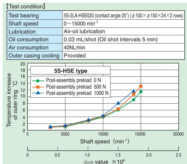
Fig. 9.25 Relationship between preload and temperature increase
