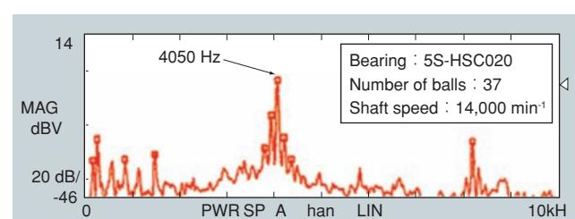
Fig. 8.12 Frequency characteristics of bearing noise (standard nozzle)
