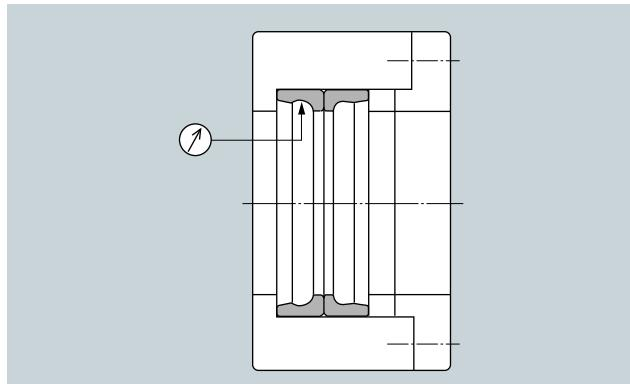
Fig. 6.13 Measuring position for roundness on outer ring raceway surface
