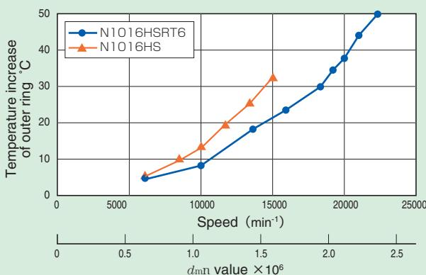
Fig. 10.13 High-speed test results (air-oil lubrication without jacket cooling)
