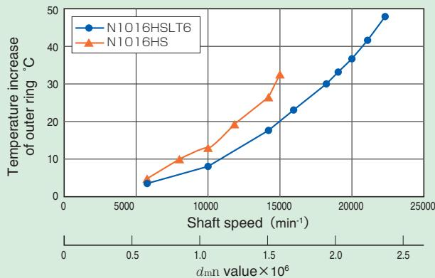
Fig. 10.16 Hgh-speed test results
