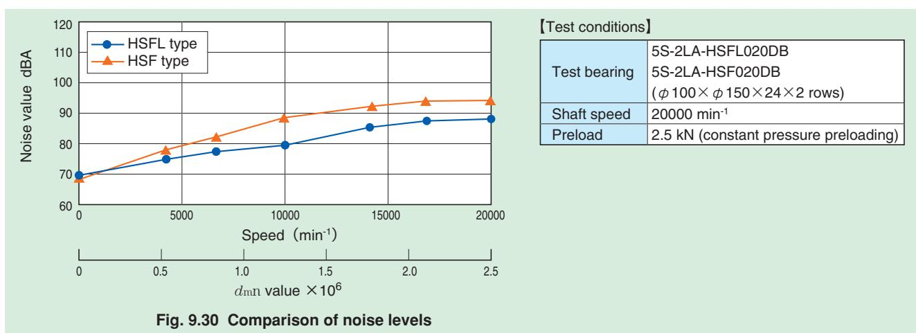
Fig. 9.30 Comparison of noise levels
