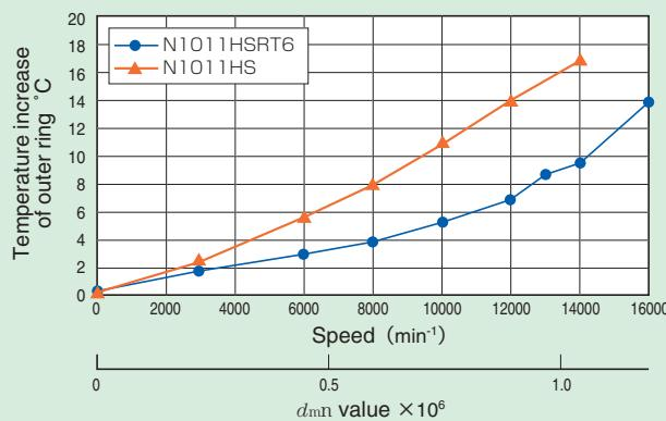
Fig. 10.11 High-speed test results (grease lubrication without outer case cooling)
