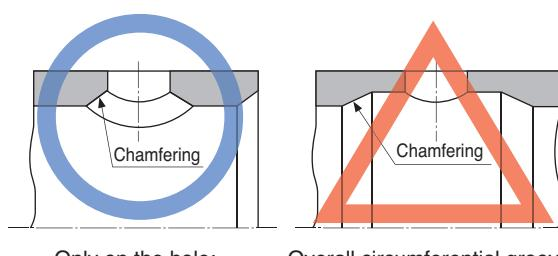
Fig. 9.35 Chamfering of re-lubricating hole on the housing
