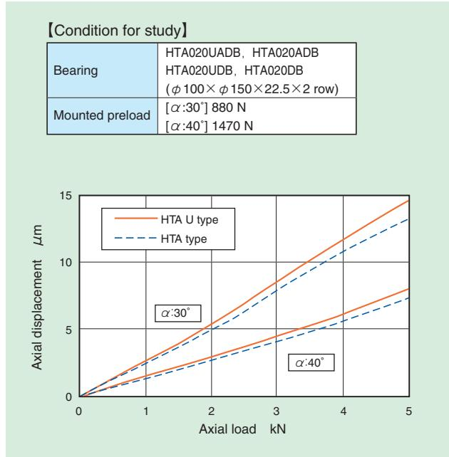
Fig. 11.3 Axial load and rigidity
