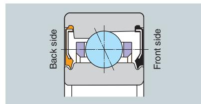
Fig. 9.8 Standard grease-lubricated sealed angular contact ball bearings
