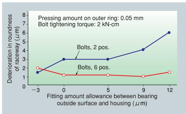
Fig. 6.14 Effect of fit of outer ring on roundness of raceway surface
