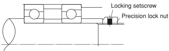
**Fig. 6.9** Tightening with precision bearing nut
