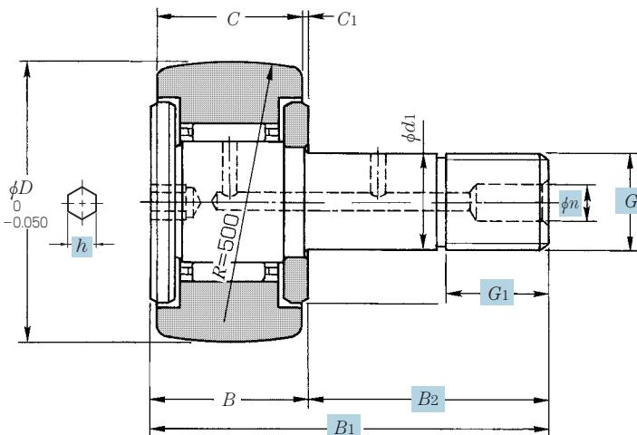
The dimensions of standard cam followers (marked with in the diagram above) are different from those of NTN pallet changer cam followers. Please see the reference dimensions in the table below.
