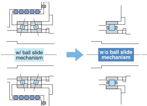
Capable of replacing angular contact ball bearings up to  $d_{mn}$  value of 2,300,000 [air-oil lubrication] or 1,150,000 [grease lubrication].
