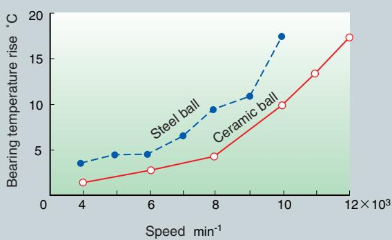
Fig. 9.15 Comparison of temperature rise between bearings with ceramic balls and those with steel balls
