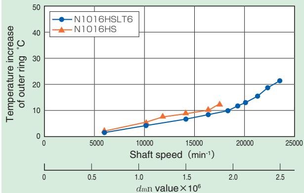
Fig. 10.17 High-speed test results
