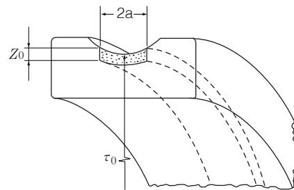
Fig. 3.1 Stress volume resulting from rolling contact according to L-P theory
