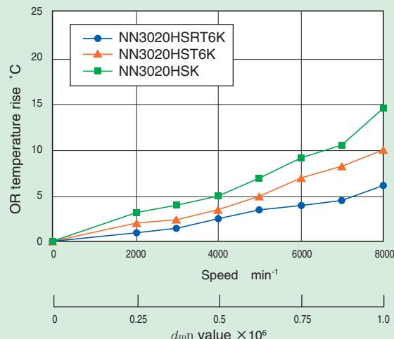
Fig. 10.5 Comparison of temperature rise (grease)
