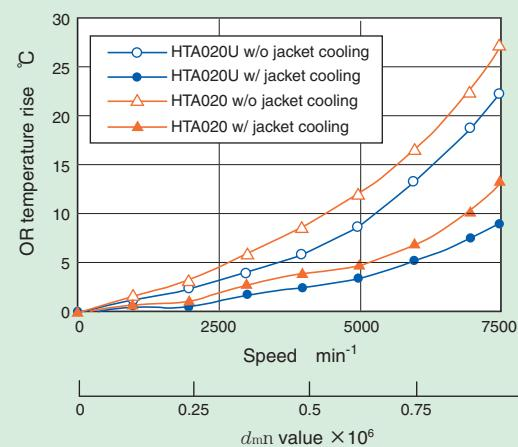
Fig. 11.8 Comparison of temperature rise (Air-oil,  $\alpha=40^\circ$ )
