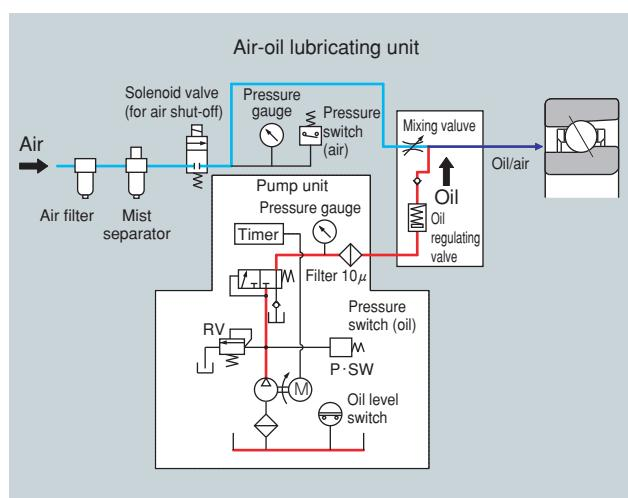
**Fig. 7.2** Air-oil lubricating system
