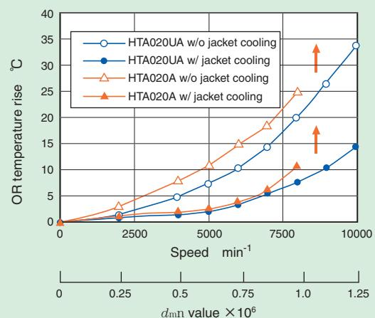
Fig. 11.6 Comparison of temperature rise (Air-oil,  $\alpha=30^\circ$ )
