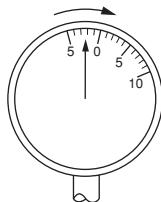
**Fig. 6.28 Adjustment for positive clearance (remaining internal clearance: +1.0 μm)**
