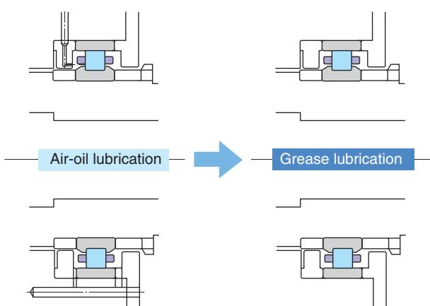
Capable of replacing air-oil lubricated bearings up to  $d_{mn}$  value of 1,150,000.
