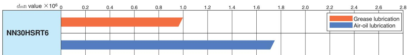
Notes) Permissible speed of each bearing ( $d_{mn}$  value) varies depending on the specifications of the machine for which the bearing is used (motor drive system, cooling system, and construction around the bearing). Consider the optimal choice referring to the above guideline and contact NTN.
