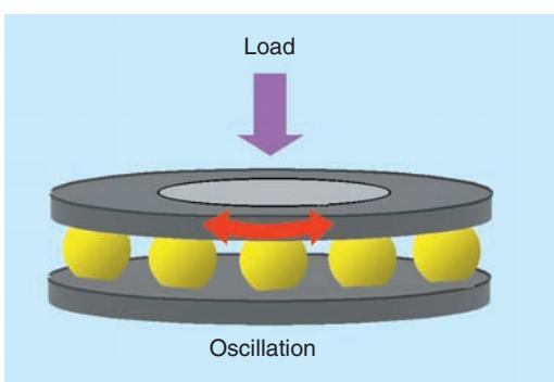
**Fig. 13.5 Fretting resistance test (rolling)**
