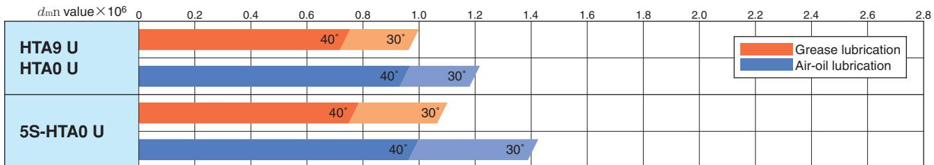
Notes) Permissible speed of each bearing ( $d_{mn}$  value) varies depending on the specifications of the machine for which the bearing is used (motor drive system, cooling system, and construction around the bearing). Consider the optimal choice referring to the above guideline and contact NTN.
