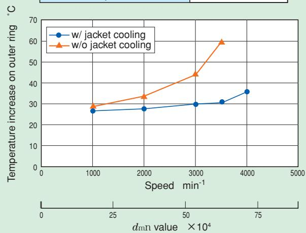
Fig. 5.7 Variation in bearing temperature depending on presence/absence of jacket cooling (cylindrical roller bearing)
