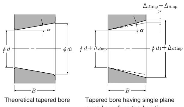
Tolerance of 1/12 taper angle  $4^{\circ}46'18.8''_0^{+24''}$
