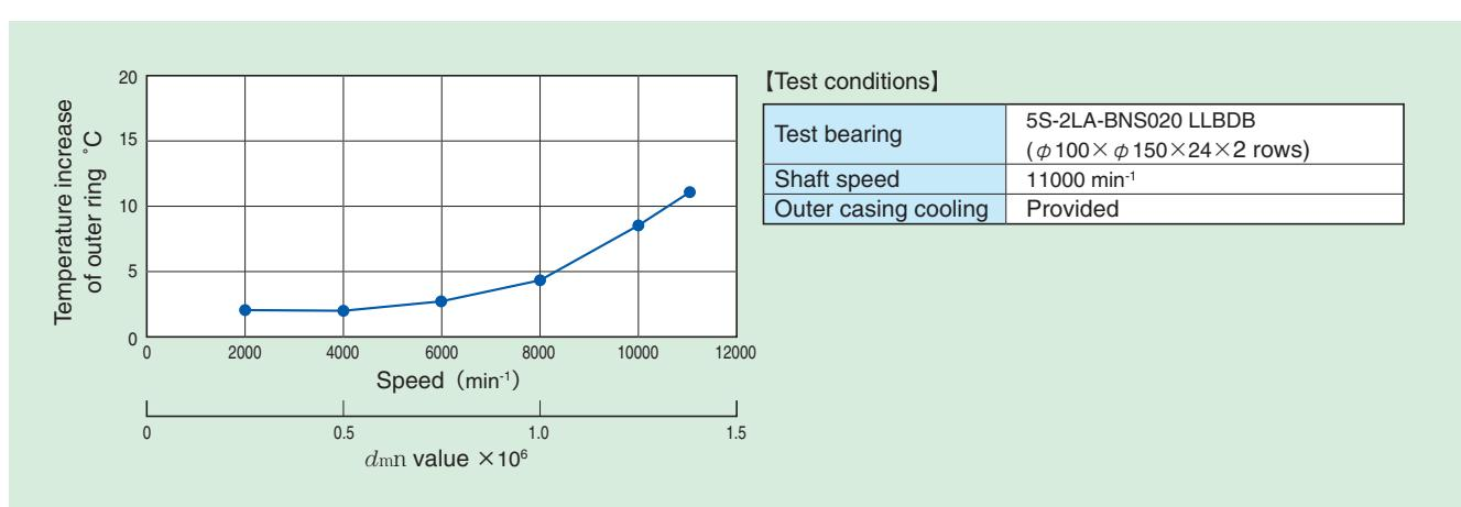
Fig. 9.45 High-speed test results
