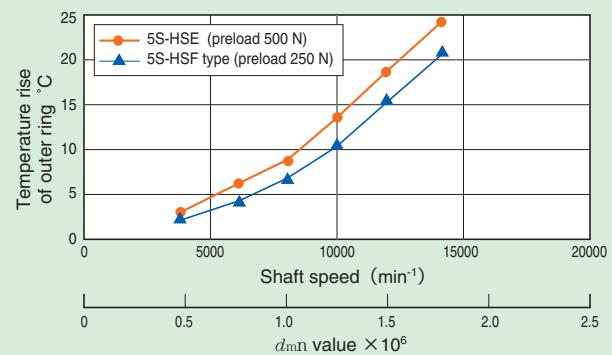
Fig. 9.28 Comparison of temperature rise
