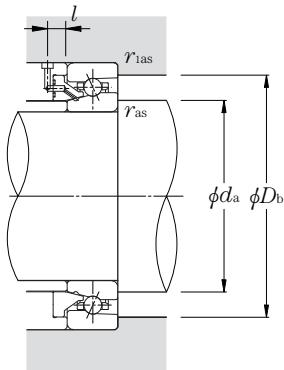
**Dynamic equivalent radial load**  $P_r = X F_r + Y F_a$
