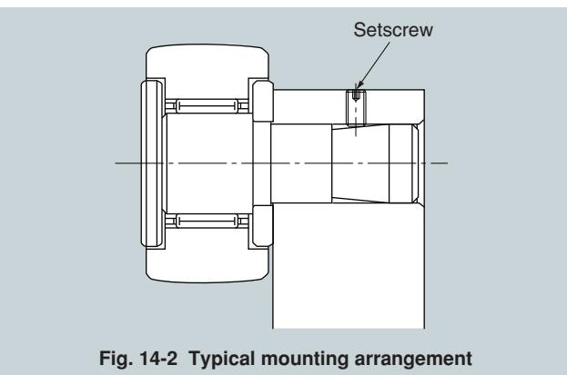
Fig. 14-2 Typical mounting arrangement
