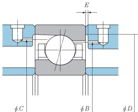
Fig. 7.5 78C, 79C, 70C and 72C types
