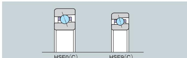
Fig. 9.3 High-speed angular contact ball bearings
