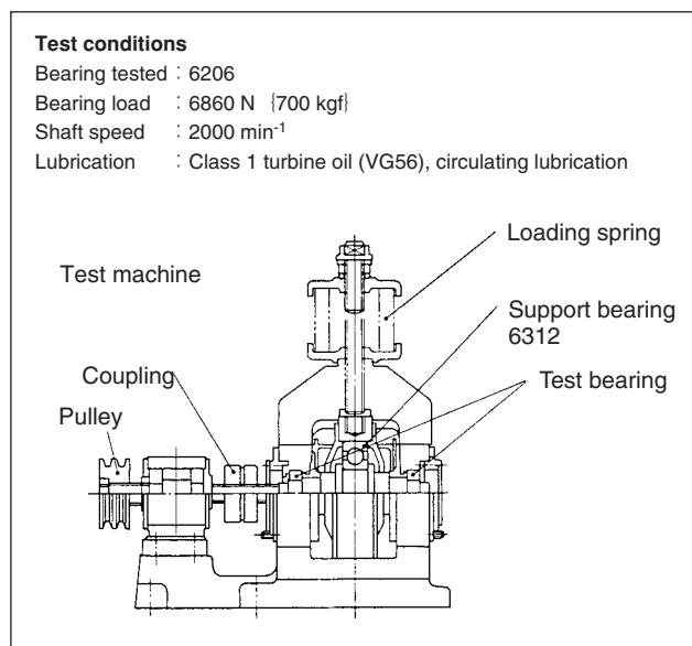
Fig. 9.17 Radial load-type bearing life test machine
