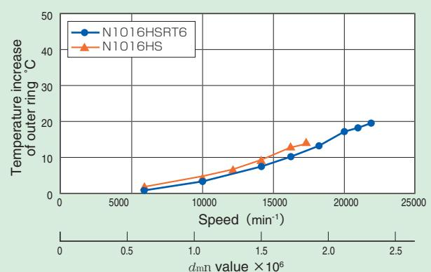
Fig. 10.14 High-speed test results (air-oil lubrication with jacket cooling)
