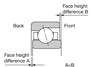
Fig. 9.13 Flush grinding
