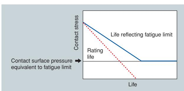
Fig. 3.3 Basic concept of fatigue limit
