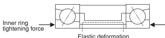
Fig. 6.11 Elastic deformation of inner ring spacer
