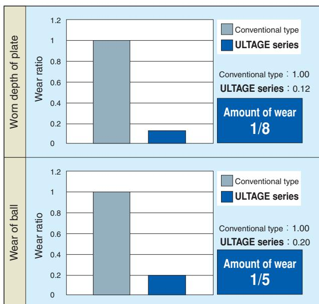
Fig. 13.4 Ratio of fretting corrosion in sliding mode
