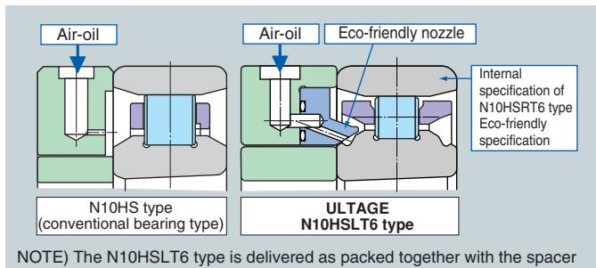
NOTE) The N10HSLT6 type is delivered as packed together with the spacer with the eco-friendly nozzle. The bearing type code N10HSLT6 represents the bearing proper, while a spacer code stands for an eco-friendly nozzle proper or a spacer having a built-in nozzle. For more details, see "3 Bearing Designations".
