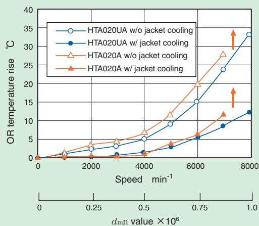
Fig. 11.5 Comparison of temperature rise (Grease,  $\alpha=30^\circ$ )
