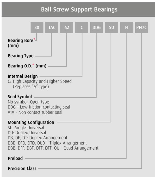
\* For inch series bearings, the fractional portion of the size is omitted.
