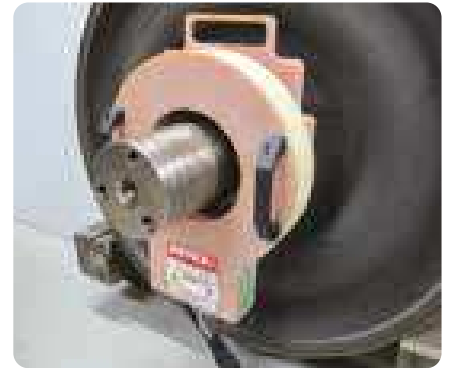
Heating labyrinth rings for dismounting
