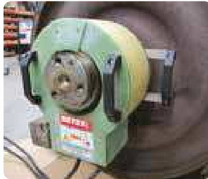
Heating bearing rings for dismounting
