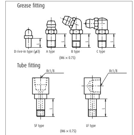
Fig. 12 Grease fitting and tube fitting
