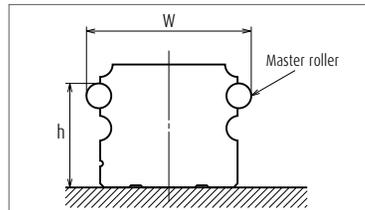
Fig. 4 Measuring groove accuracy
