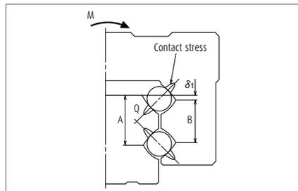
Fig. 2 Enlarged illustration: Offset Gothic arch
