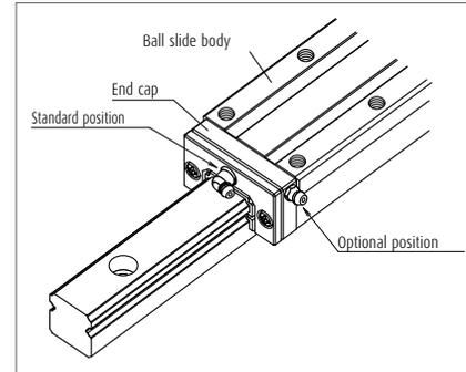
Fig. 13 Mounting position of lubrication accessories
