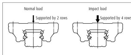
Fig. 3 When load is applied
