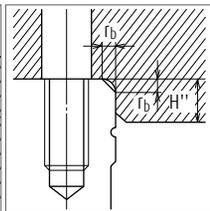
Fig. 11 Shoulder for the ball slide datum surface
