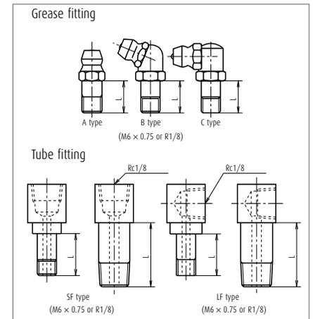
Fig. 12 Grease fitting and tube fitting
