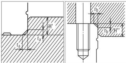
Fig. 10 Shoulder for the rail datum surface
