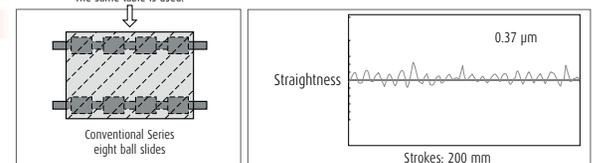
Fig. 6 Measurement results of HA Series and conventional Series
