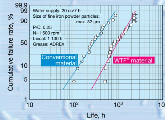
Figure 4. Trial usage results of WTF bearings in an actual cold rolling mill
