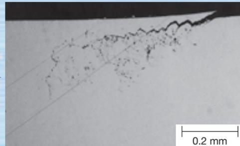
Photo 3. Cracks develop from below the surface
