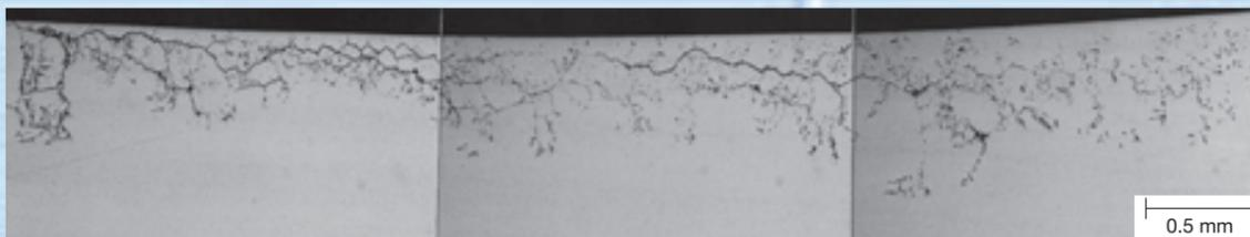
Photo 4. Cracks along grain boundary
