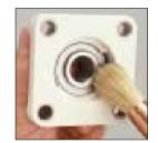
Install the shaft by mounting the bearing unit housings on the supporting frame. Tighten the inner ring retaining screw to the required torque indicated in the torque value table. (see page 14)
