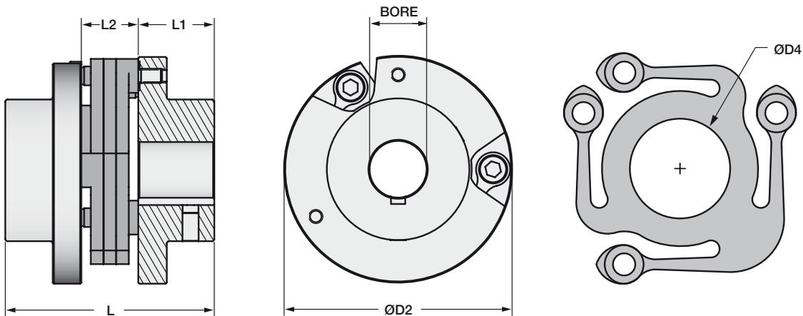
The above drawing is valid for C030P, C060P and C075P. C045P will still use the triangular style hubs. Consult factory if necessary.
