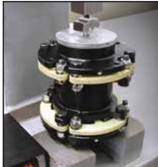
Coupling Axial Stiffness Test
