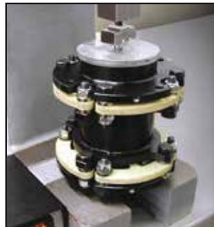
Coupling Axial Stiffness Test
