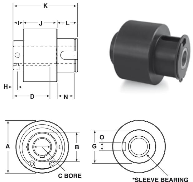
\*The ID of the sleeve bearing will be sized to match the C Bore. When ordering this option, only specify one bore.
